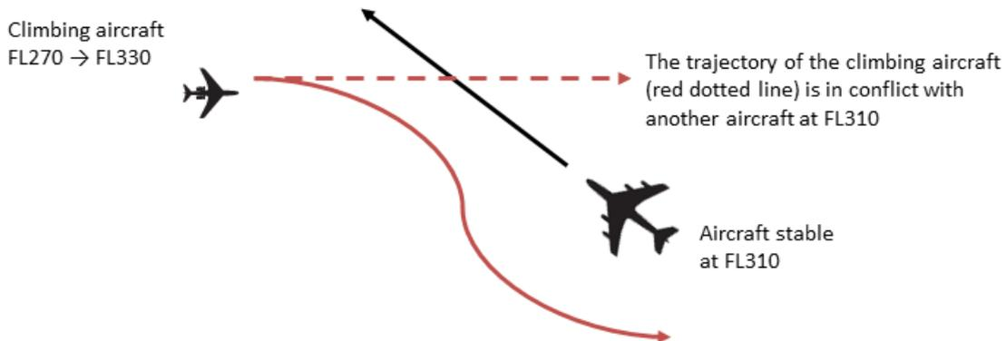
The controller may separate the two aircraft providing radar vectors or a direct route on a point in order to avoid level flight to the climbing aircraft.
