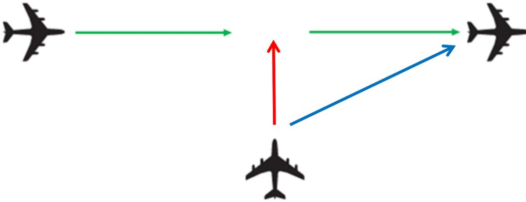
In the example above, if ATC gives to the aircraft the instruction to join the route with a clearance like the **red arrow**, the situation will be problematic as there is a flight time to join the route and the final result can be a possible loss of separation or a bad regulation on route (see figure below).
