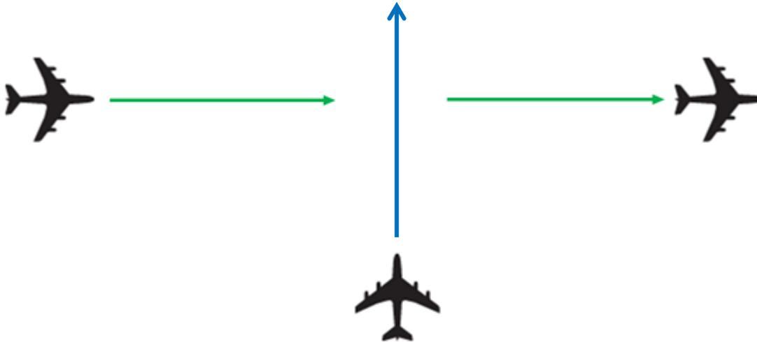
Cleared flight level shall be issued and reached 15NM minimum before the crossing time at the latest.
