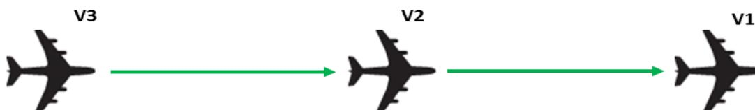
To maintain the required separation, speed clearances shall be issued in order to reach the following hierarchy:  $V1 \geq V2 \geq V3$
