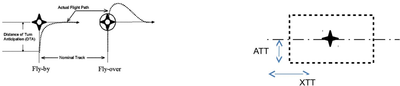
Along a RNAV flightpath, a turn between two segments will require a minimum segment length to make sure aircraft will have time to be stabilized, in particular between fly-over waypoints.
