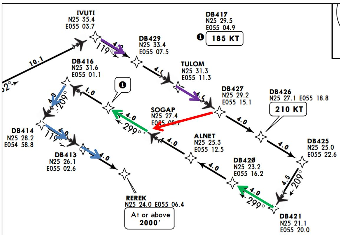
On the sequence above the red arrow shows how to optimize the traffic regulation flow by inserting an aircraft between two others with a sufficient available space (between aircraft at **SOGAP** and aircraft at **DB421**).
