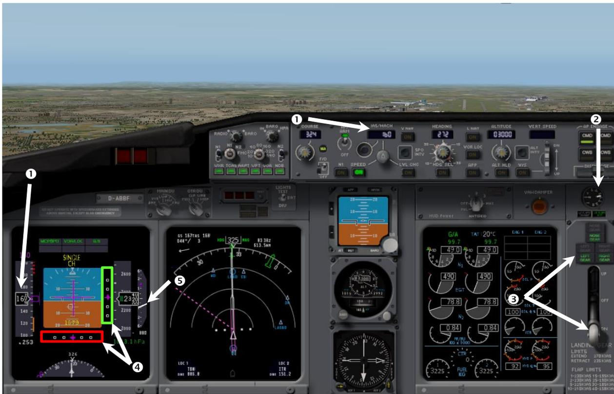
When localizer and glide path indicator are located near the middle of the indicator, you can consider the ILS being established.
