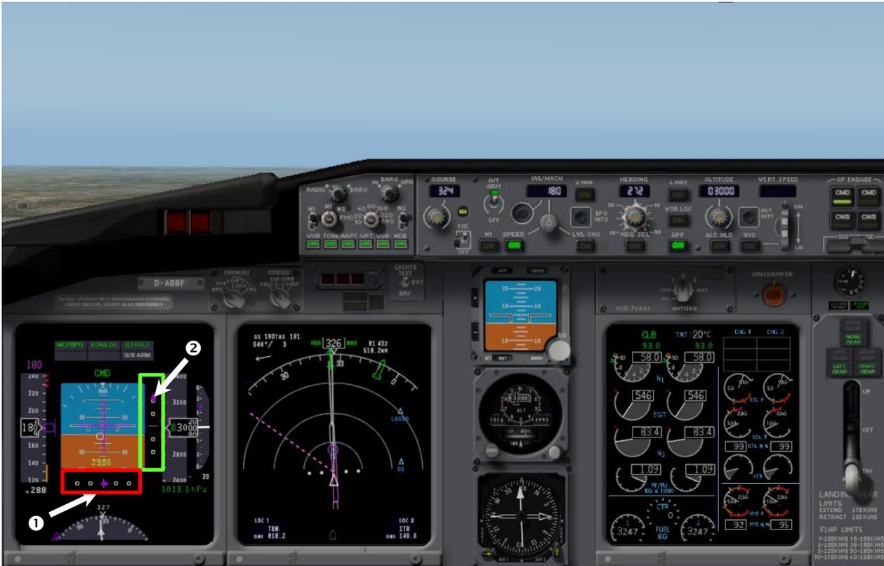
When the glide indicator is on the top it means that the glide path is above the aircraft or the aircraft is below the glide path.
