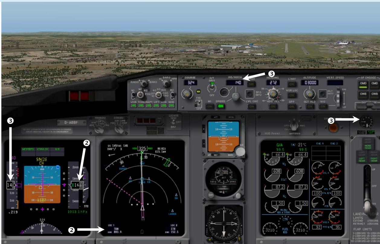
When the descent rate is stabilized, the approach speed should be reduced to the final approach speed.
