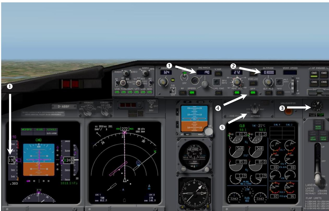
When the localizer indicator is on the left it means that the localizer path is on the aircraft's left, or the aircraft is on the right of the localizer path.
