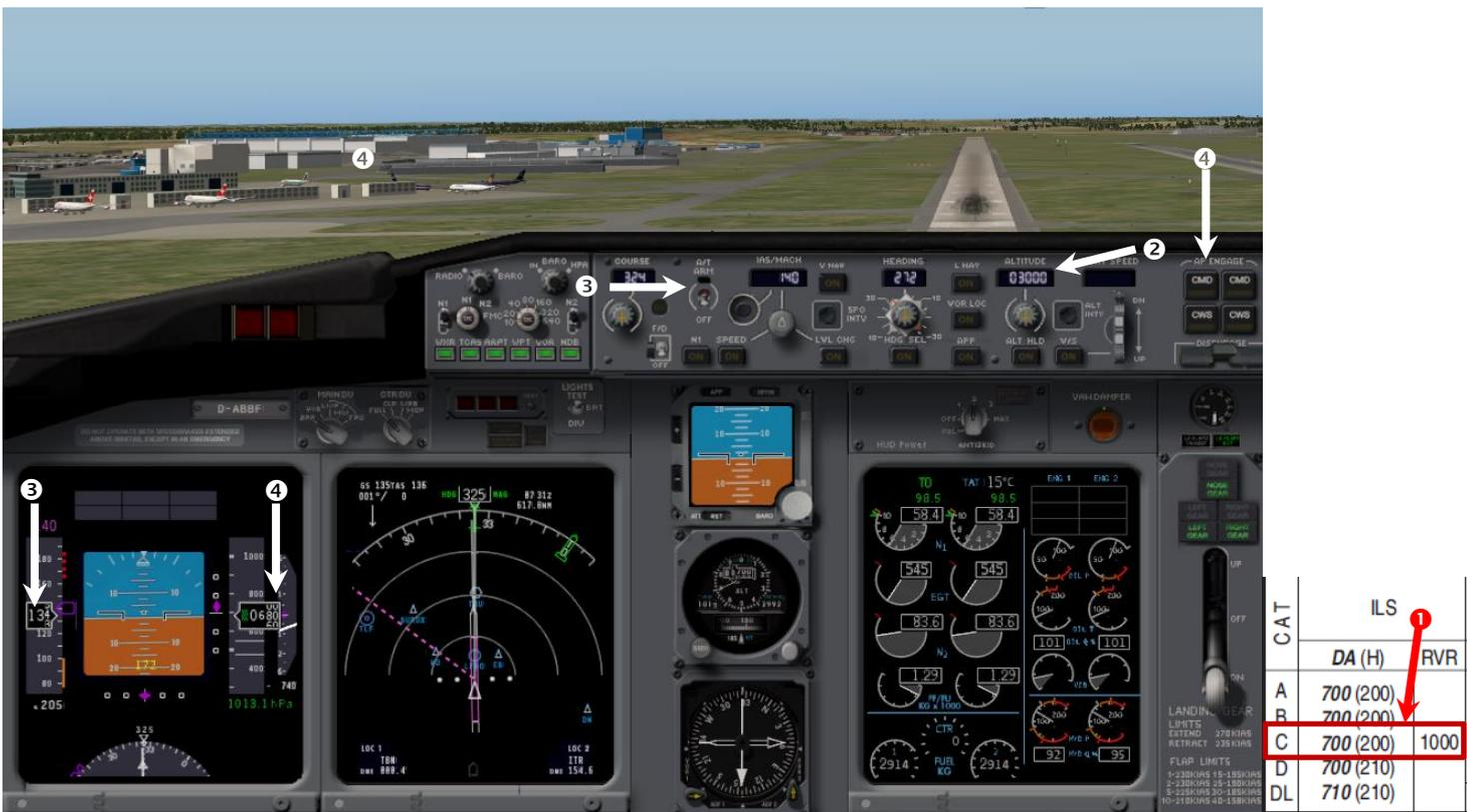
The aircraft must be stabilized on final in landing configuration at least 1000 ft above the ground. The pilot in command shall not hesitate to go around if his aircraft is not stabilized on final, or the approach speed is excessive.
