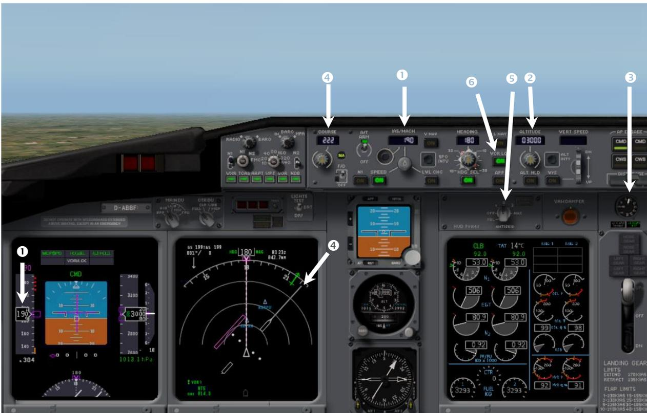
If you are far from the VOR Radial, the VOR indicator is set to maximum deviation and remains at this position (like the image hereabove). If you are close to the path, the indicator will move to the central position.
