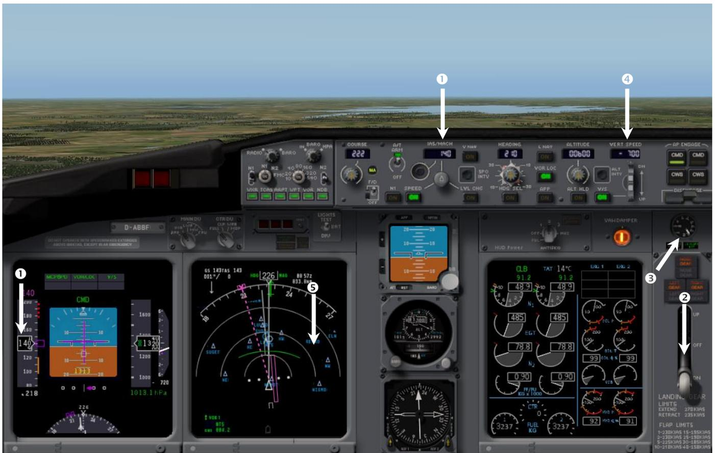
In the example above, the aircraft is below the target altitude within the altitude tolerance (<100ft)
