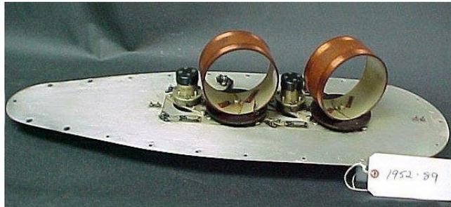
The NDB transmits signals in all directions that reach airborne ADF's loop and sense antennas. When both inputs are processed together, the equipment is able to display the relative bearing on the indicator instrument.
