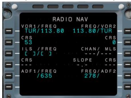
Figure: example of a frequency selector located in FMC
