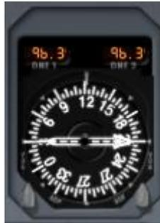
Figure: Dual RMI of airbus aircraft
