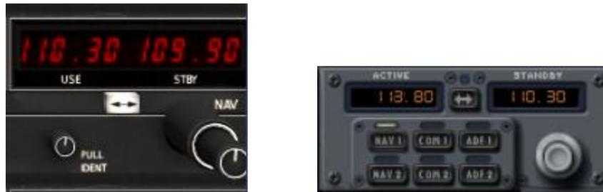
Figures: 2 examples of a DME/NAV frequency selector:
