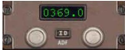
ADF selector on a Boeing radio panel
