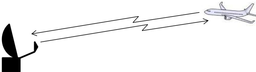
The time difference between the pulse emission and the reflected wave reception is proportional to the distance of the target with respect to the emission antenna. The position of the antenna at the reception, corrected by the fact the antenna is continuously turning, is linked to the azimuthal angle of the target.
