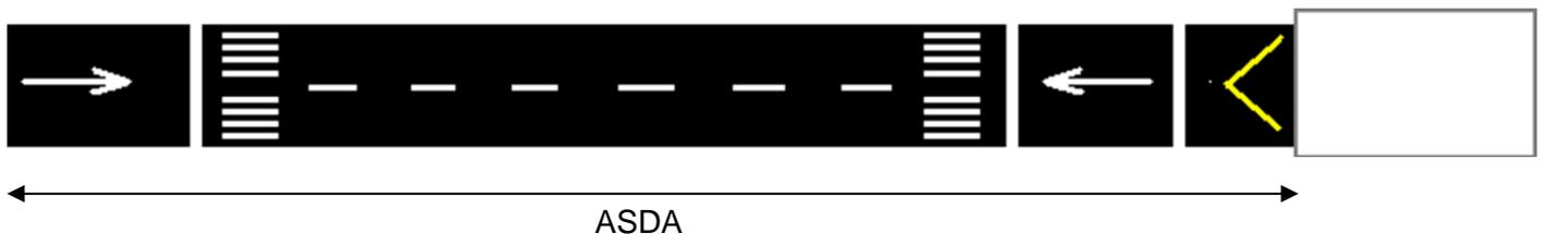
ASDA is the maximum run distance for an aircraft when performing a rejected take-off.
