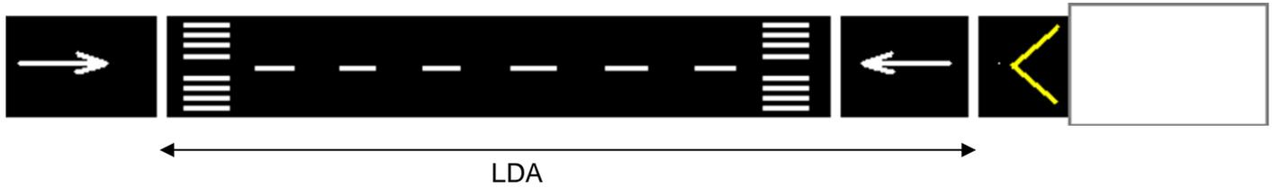
LDA never includes runway section before displaced threshold before touchdown point.
