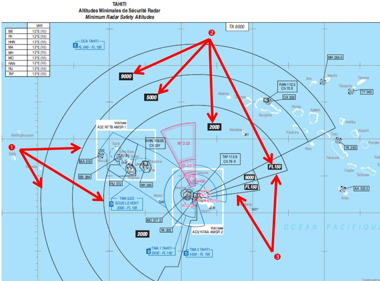
MVA description chart at NTAA named Minimum Radar Safety Altitudes
