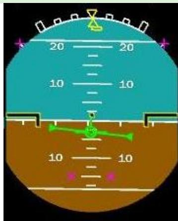
Usually, most airlines require that the flight director must be turned off when using the FPV.
