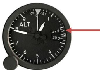
Example of an altimeter with the setting displayed in inches of Mercury
