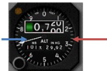
Example of an altimeter showing both units of setting: (red = inHg ; blue = hPa)
