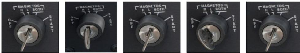
When running on a single magneto, do not allow more than 125 RPM drop. Also, the lowest value differential between the two magnetos must not exceed 50 RPM.
