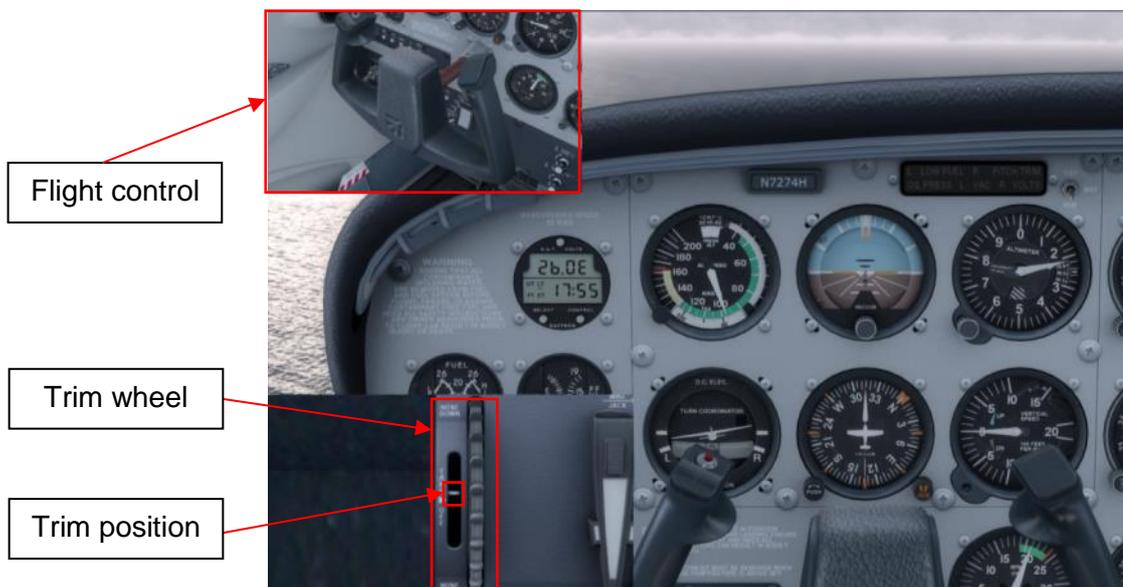
Only to illustrate the powerful advantage of trimming the aircraft, we can see for example that a full deflection of the control surface can be countered by the trim.
