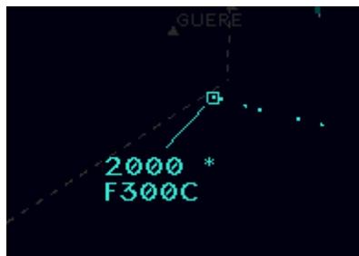
Figure showing aircraft squawking 2000 in non-controlled area after ATC transfer to Unicom.
