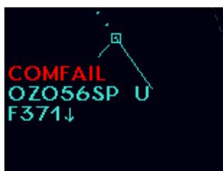
A controller, who notices a communication failure code, will determine the extent of the failure by instructing SQUAWK IDENT or to change the code. With that operation, if it is determined that the aircraft receiver is functioning, further control of the aircraft will be continued using code changes or IDENT transmission to acknowledge receipt of clearances.
