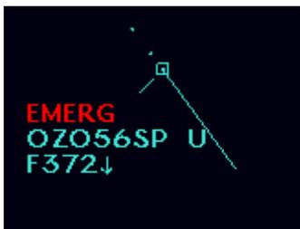
Radar capture with aircraft using active code 7700
